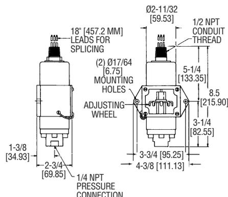
Series 1000E explosion-proof also available in 1000EH explosion-proof, hermetically sealed switch assembly.
